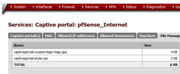
Fig. 9 Adding Files Needed for Login and Error Page
