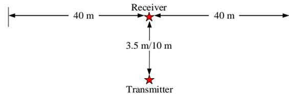
**Fig. 2 Sketch of the Setup for collecting RF Propagating Data at Roadway**
