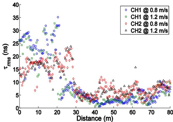
**Fig. 8 RMS Delay Spread Versus Distance for Ch1 and Ch2**
