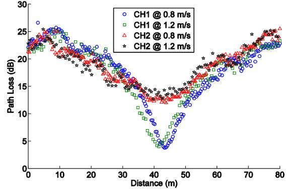
Fig. 5. Scatter Plots of the Path Loss versus Distance for Channels CH1 and CH2
