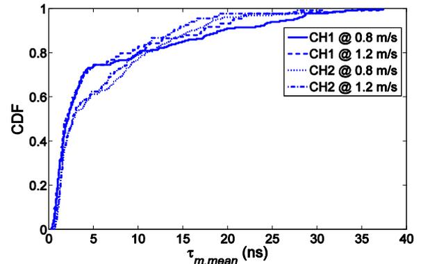
**Fig. 7 Cumulative Distribution Function versus Mean Excess Delay Spread for CH1 and CH2**
