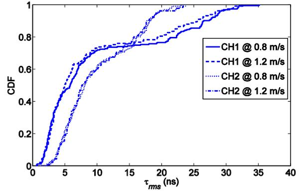
**Fig. 6 Cumulative distribution function versus RMS delay spread for CH1 and CH2**
