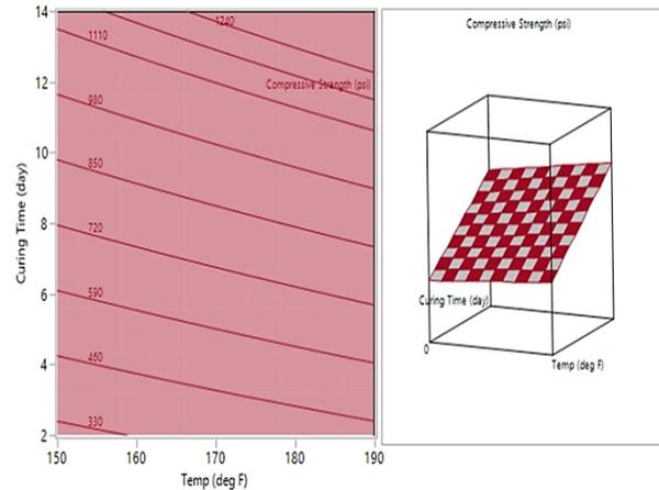
**Fig. 7 Surface Response Plot for Compressive Strength Model**
