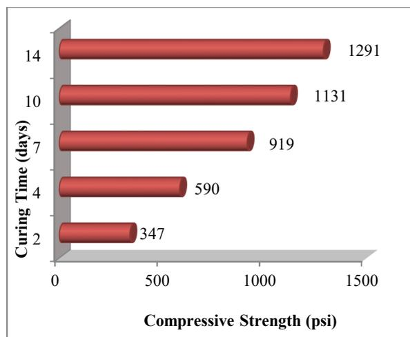
Fig. 2 Effect of Curing Time on Compressive Strength at 190 °F (87.8 °C)
