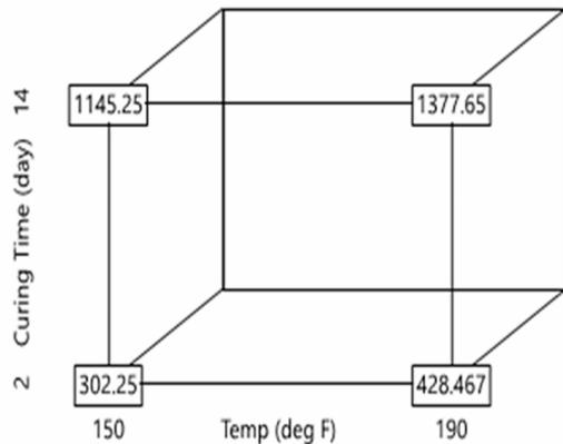
**Fig. 5 Cube Plot for Compressive Strength Model**
