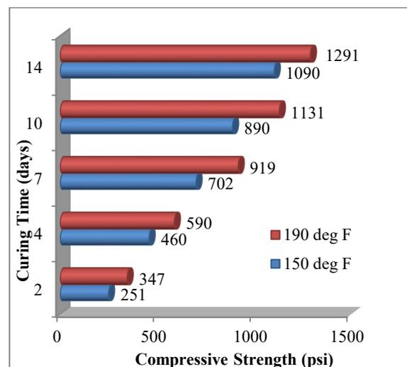
Fig. 3 Effect of Temperature on Compressive Strength
