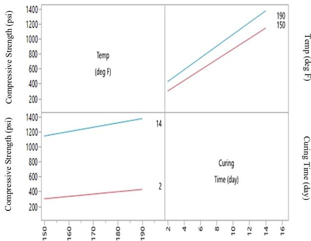
**Fig. 6 Interaction Profile for Compressive Strength Model**
