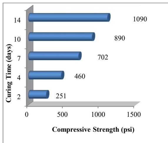
Fig. 1 Effect of Curing Time on Compressive Strength at 150 °F (65.6 °C)
