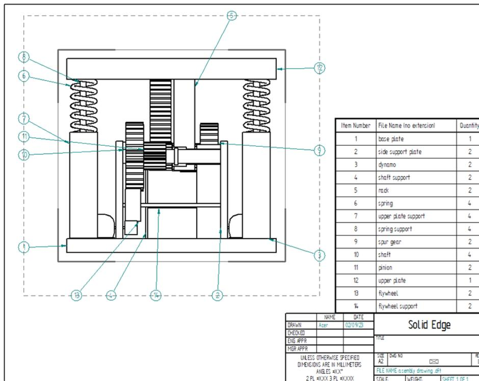
**Fig. 11 Detailed Drawing of the Proposed Design, together with the Rack and Pinion Configuration**
