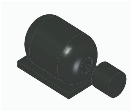
**Fig. 7 DC Generator (Dynamo)**
