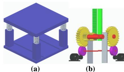
**Fig. 9 Major Mechanical Component Combinations. (a) Spring-Loaded Upper and Baseplates, and (b) Two (2) Racks with Pinions and two (2) flywheels Attached to the Ends of the two (2) Shafts Coupled with two (2) Dynamos**
