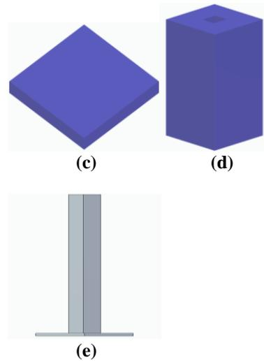
**Fig. 8 Additional Components. (a) Inner Support Plate. (b) Base Plate (300 mm x 300 mm). (c) Upper Plate (300 mm x 300 mm) (d) Upper Plate Support Pillar. (e) Spring Support**
