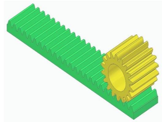
**Fig. 3 Rack and Pinion**
