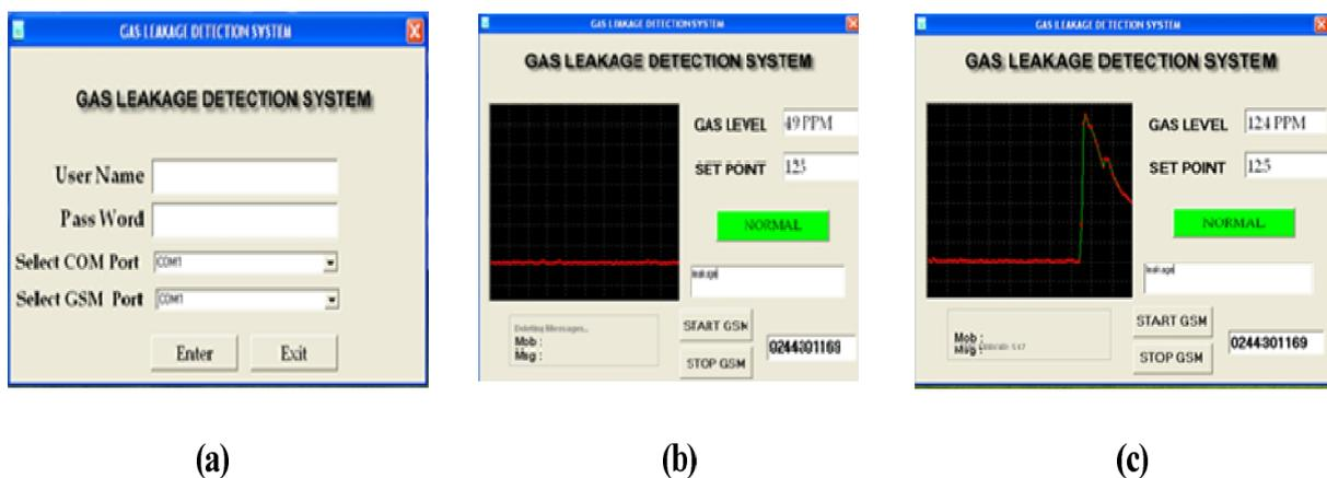
Fig. 12 (a) Login Application Software Interface, (b) Screen View before Gas Leakage and (c) Screen View after Gas Leakage
