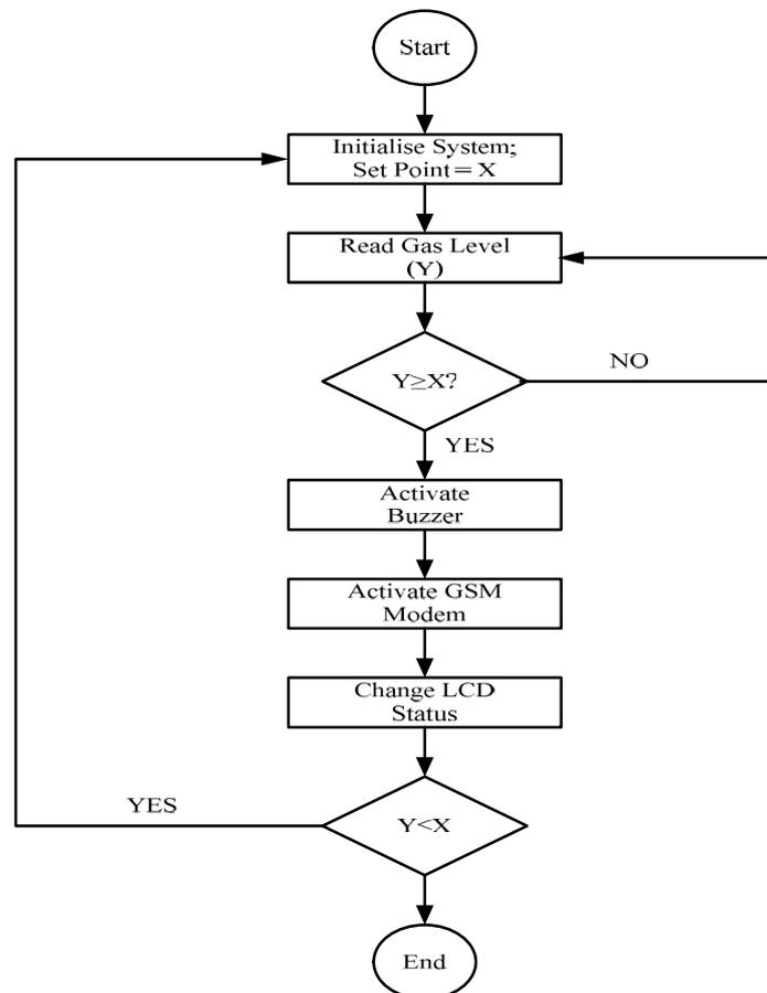
Fig. 8 Microcontroller Programming Flow Chart
