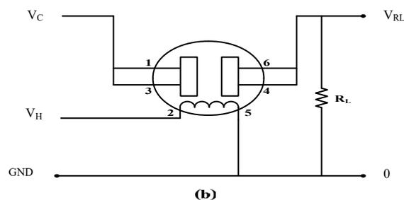
Fig. 4 (a) Structure of the MQ-5 Gas Sensor and (b) Basic Measuring Circuit of MQ-5 Gas Sensor
