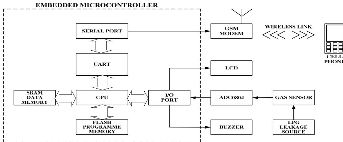
Fig. 7 Design Concept Diagram of the Proposed System
