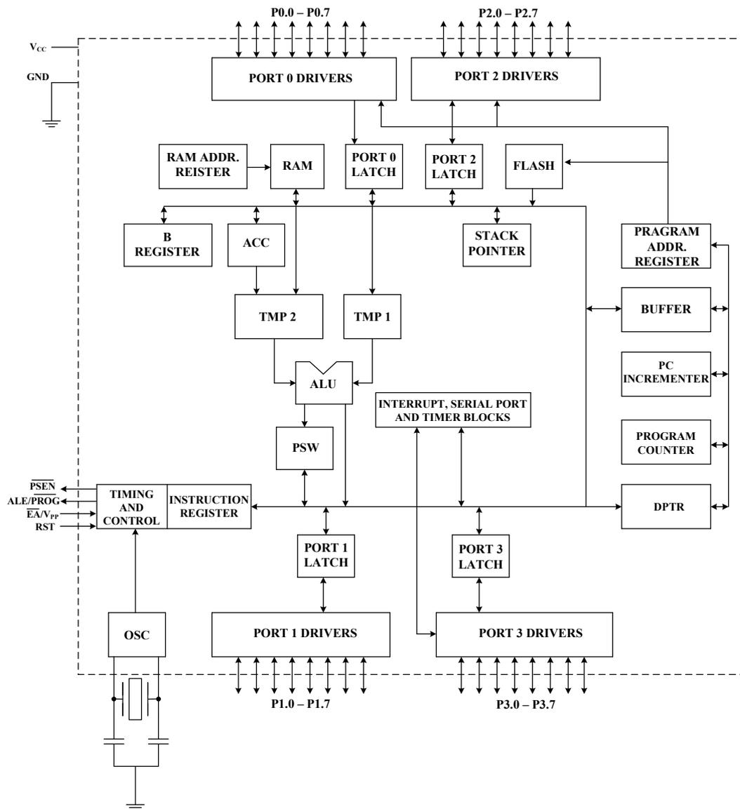
**Fig. 3 Architecture of AT89C51 Microcontroller**
