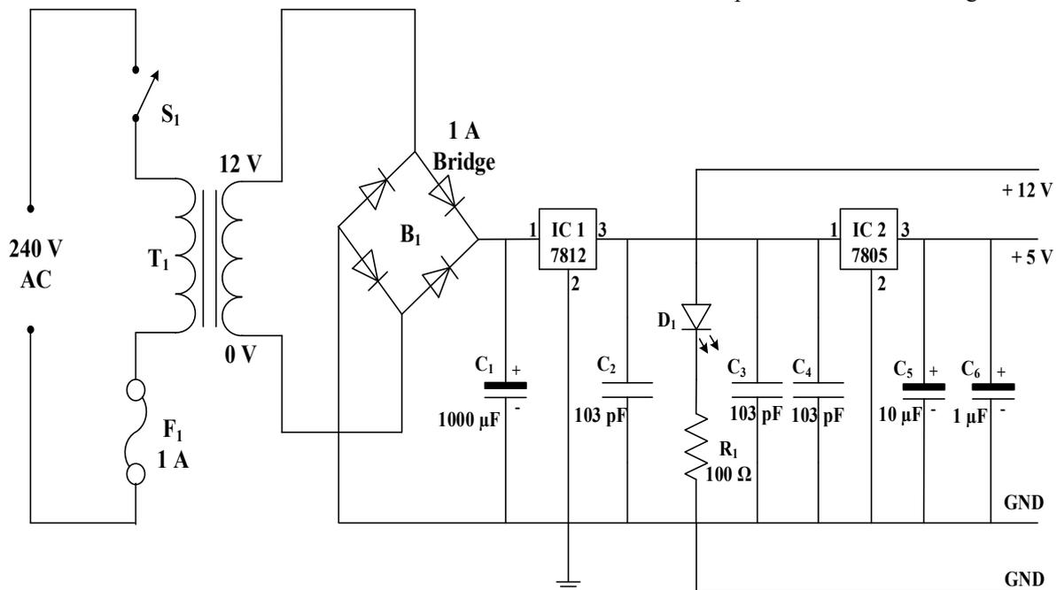
Fig. 2 12 V and 5 V Power Supply Circuit
