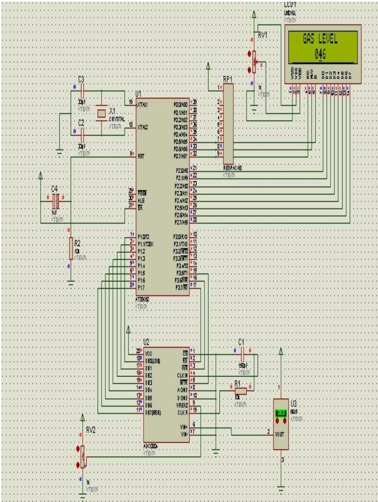
Fig. 10 Simulation Model of the LPG Leakage Detector
