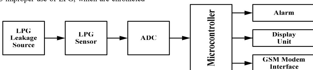
Fig. 1 Block Diagram of Proposed Design
