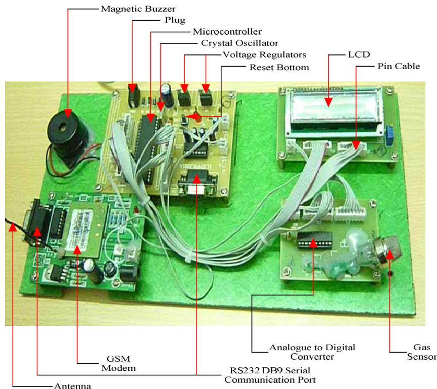
Fig. 11 Picture of the Assembled Design of the LPG Leakage Detector
