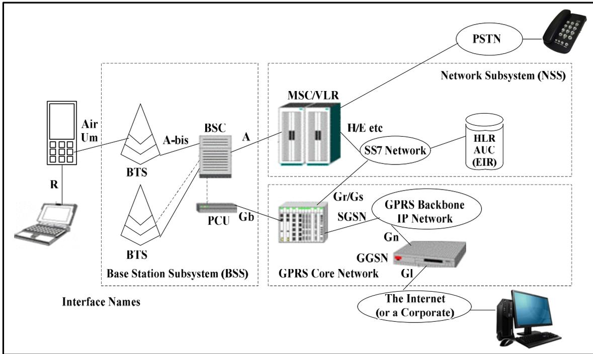
**Fig. 5 Structure of a GSM Network**
