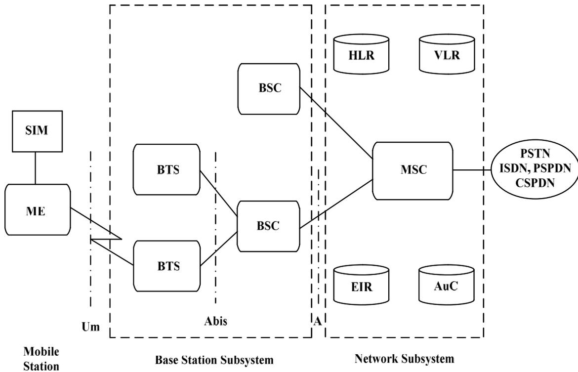
**Fig. 6 General Architecture of a GSM Network**
