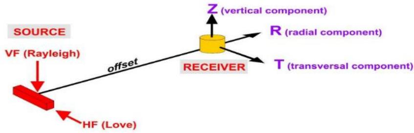
Fig. 3 Typical Acquisition Setup Depicting the Various Components of Surface Waves (Dal Moro, 2015)
