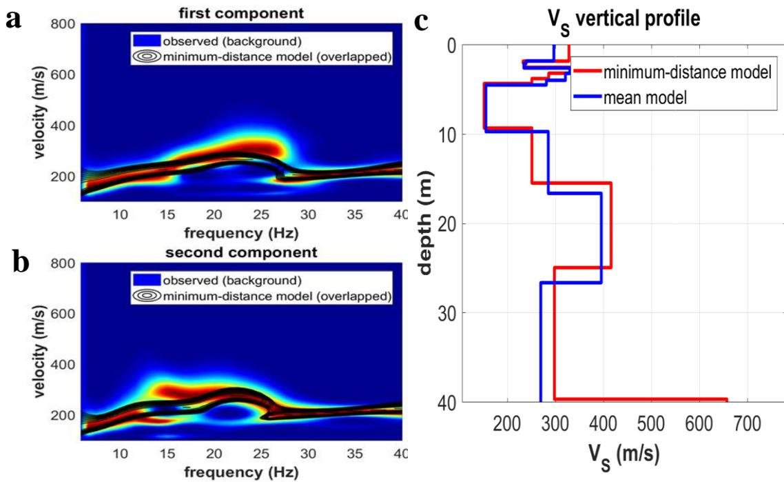
Fig. 8 Joint Inversion of Rayleigh Waves Showing Velocity Spectra for (a) Vertical Component (Z) (b) Radial Component (R) and (c) Shear Wave Velocity Profile for L300
