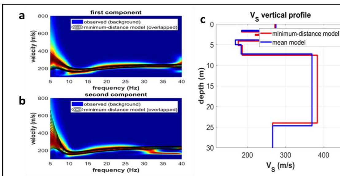
Fig. 6 Joint Inversion of Rayleigh Waves Showing Velocity Spectra for (a) Vertical Component (Z) (b) Radial Component (R) and (c) Shear Wave Velocity Profile for L100
