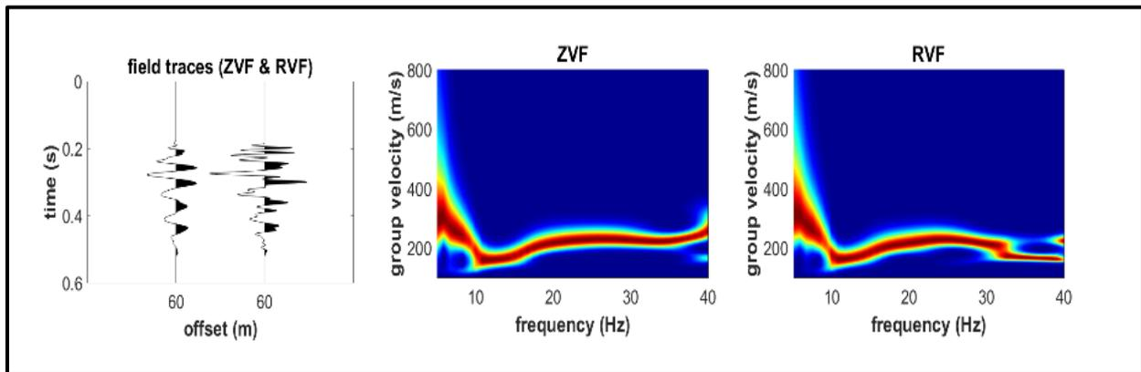
Fig. 5 (a) Seismic Traces for Vertical (ZVF) and Radial (RVF) Components (b) Group Velocity Spectra for the Rayleigh Waves
