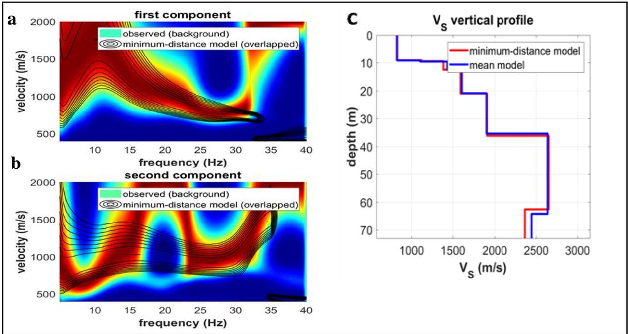
Fig. 7 Joint Inversion of Rayleigh Waves Showing Velocity Spectra for (a) Vertical Component (Z) (b) Radial Component (R) and (c) Shear Wave Velocity Profile for L200
