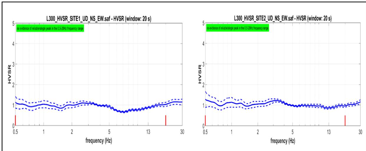
Fig. 12 Horizontal-to-Vertical Spectra Curves for L300
