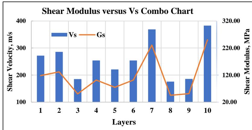
**Fig. 9 Relationship Between Shear Wave Velocity and Shear Modulus**
