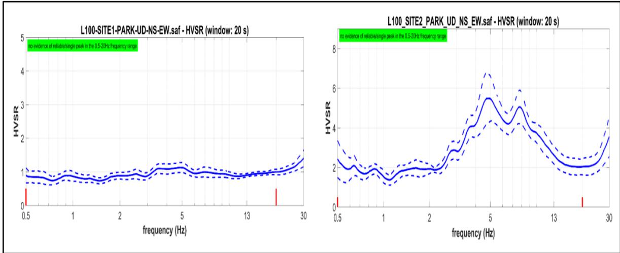
**Fig. 10 Horizontal-to-Vertical Spectra Curves on L100**
