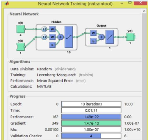
**Fig. 5 Training Process of the Artificial Neural Network Model**
