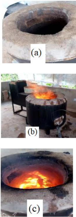
Fig. 4 Curing Operation on the Constructed Furnace
