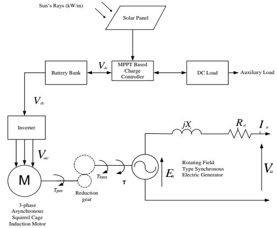
**Fig. 1 Functional Diagram of the Solar Powered Motor - Generator System**
