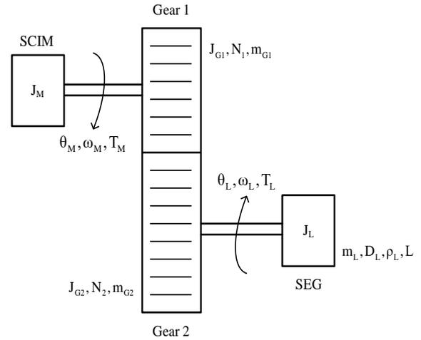
**Fig. 2 Rotational Transmission of SCIM, Gears and SEG as Load**
