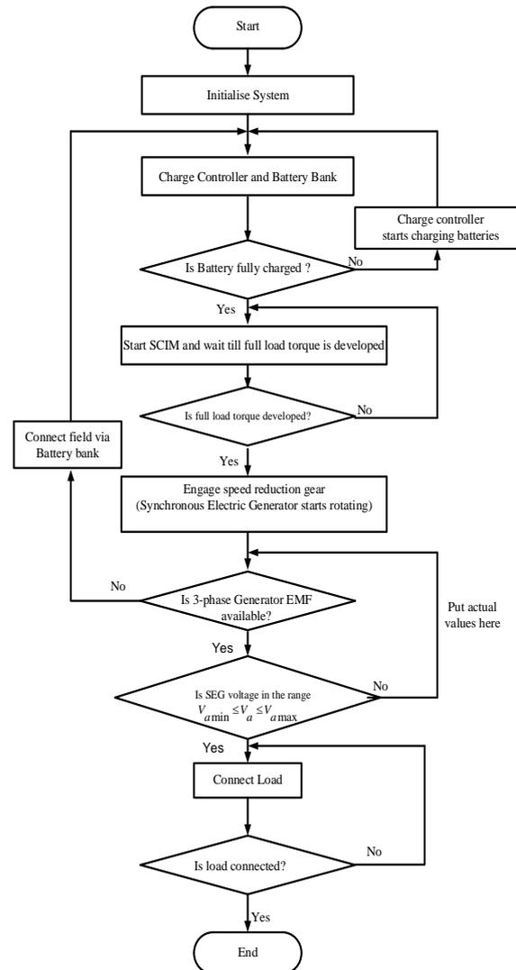
**Fig. 3 Flowchart of the Solar Powered Motor-Generator System**
