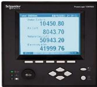
**Fig. 6 A Picture of the ION 7550 Energy Meter**
