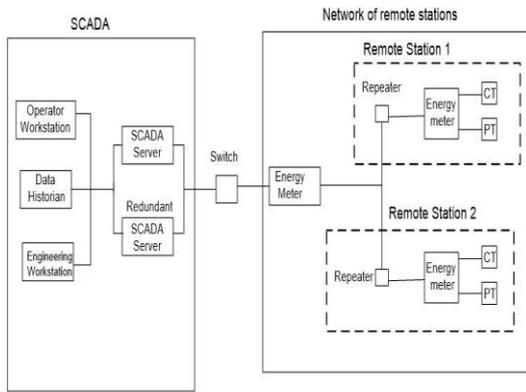
**Fig. 3 A Block Diagram of the Proposed SCADA Monitoring System**
