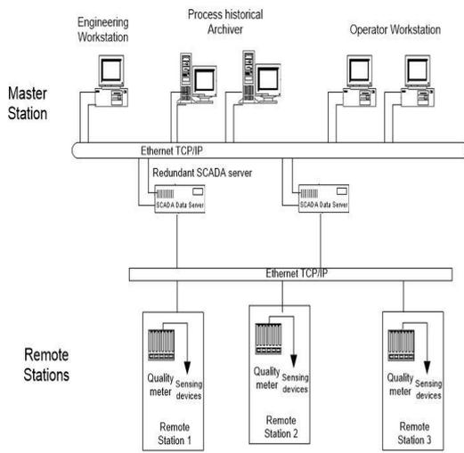
**Fig. 4 Architecture of the Proposed SCADA Monitoring System**
