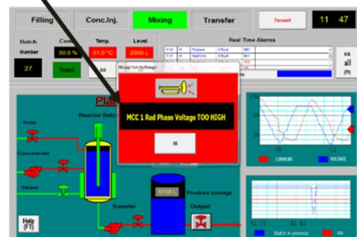
Fig. 11 A Simulation Result Showing the Fault Indication Display
