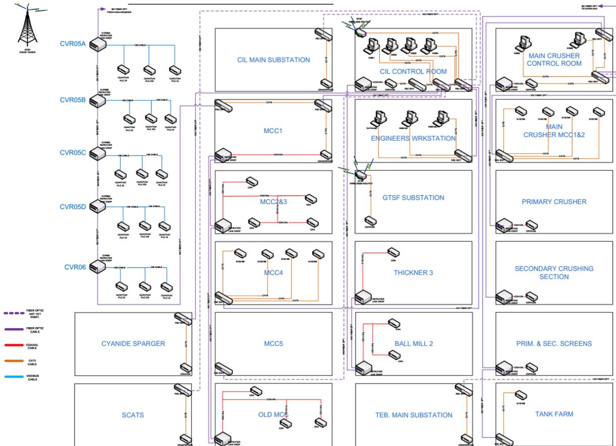
Fig. 2 A SCADA System Topology of the Gold Mine
