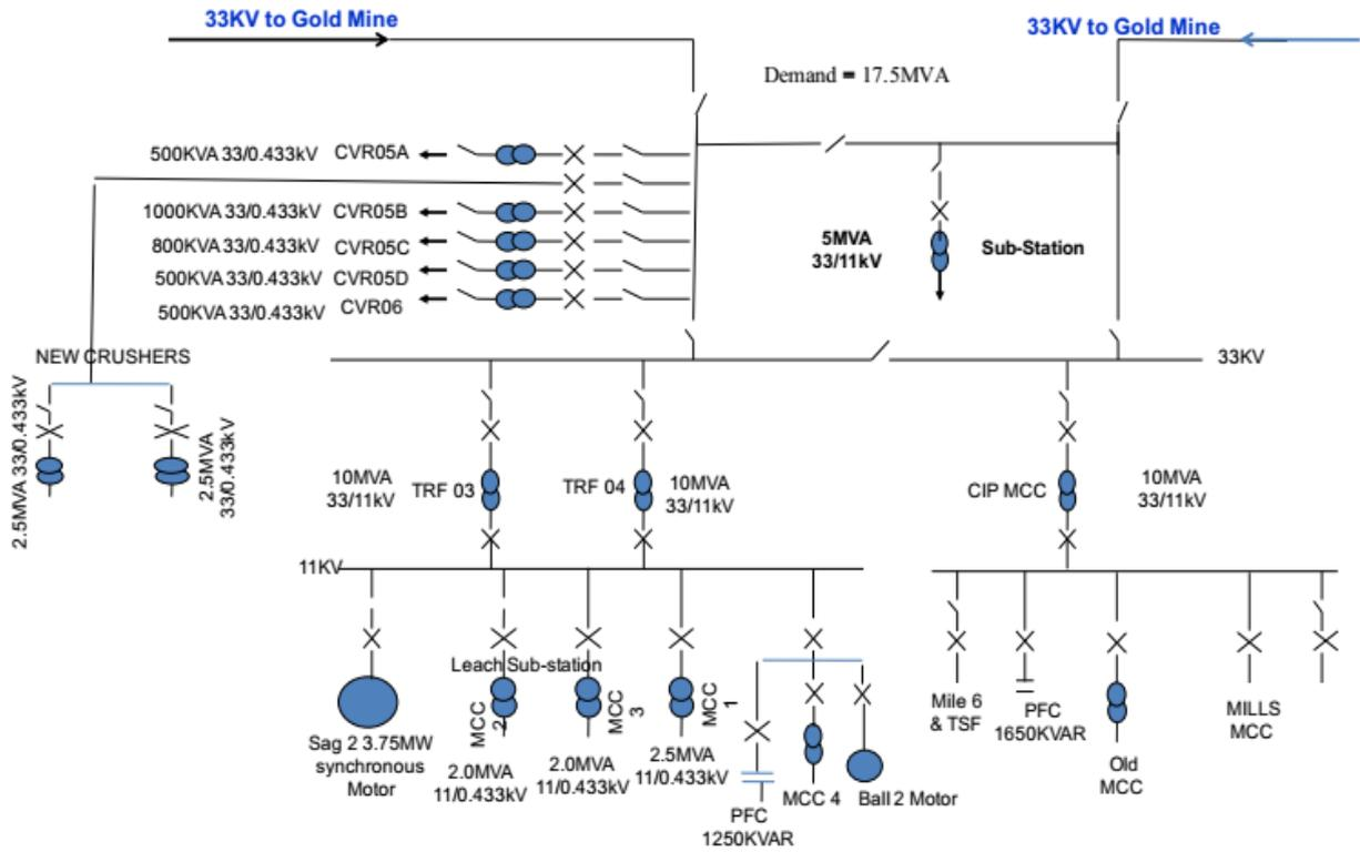
Fig. 1 Power Distribution Network of the Gold Mine
