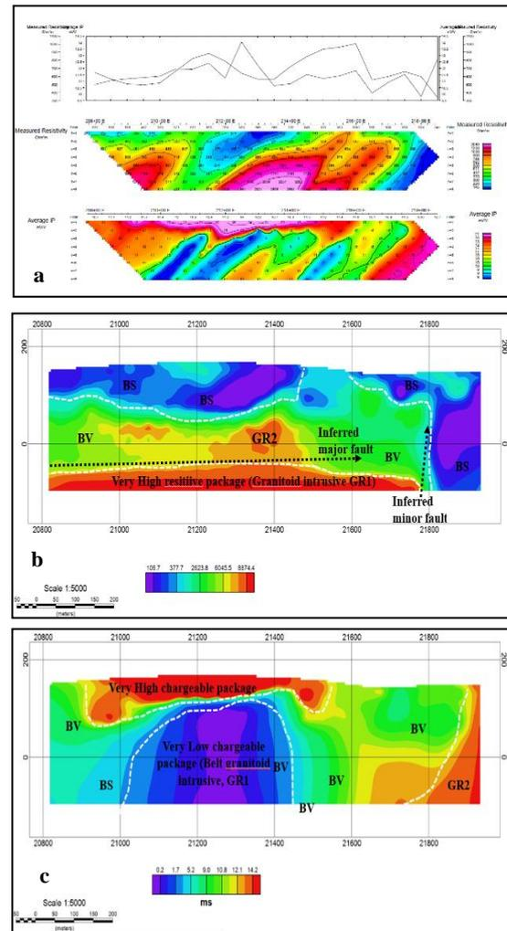
**Fig. 7 (a) Pole-Dipole Pseudo-Section, (b) Resistivity and (c) Chargeability Model Inversions. Section L22700 North**
