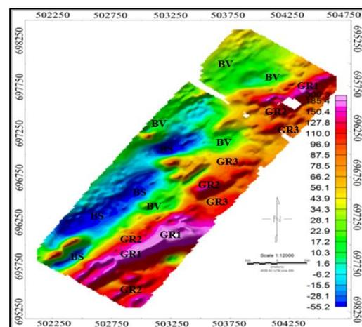
**Fig. 3 Reduced-to-Pole Anomaly Showing Interpreted Lithological Units**
