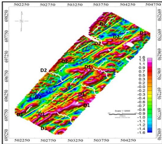
**Fig. 4 Tilt Derivative Anomaly Showing Structural Lineament**
