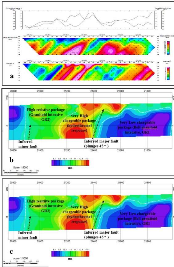
**Fig. 6 (a) Pole-Dipole Pseudo-Section, (b) Resistivity and (c) Chargeability Model Inversions. Section L21500 South**
