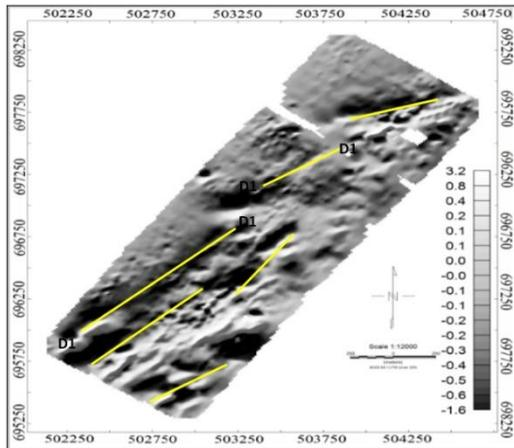
**Fig. 5 1VD Anomaly and Structural Lineament**
