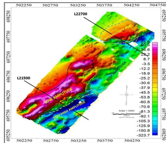
**Fig. 2 Total Magnetic Intensity (TMI) Grid Map Showing Pole-Dipole Section Profiles**
