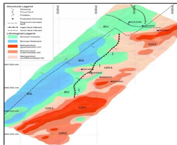
**Fig. 8 Mineral Prospectivity Map Showing Structural Features and Proposed Drill**
